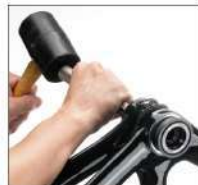
3. Tap the Cup out with A Hammer
